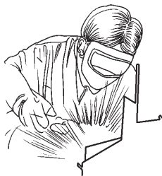
A worker uses an oxy-acetylene torch to do some welding.
